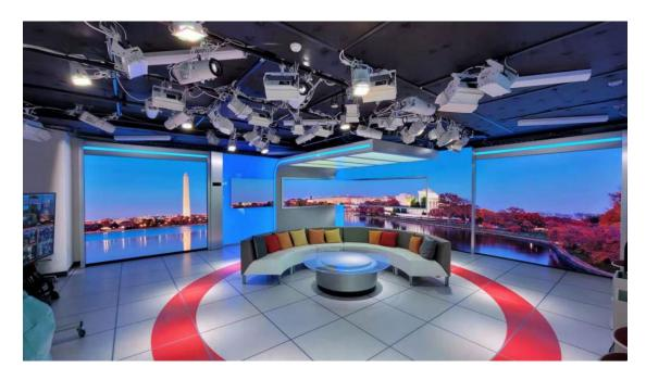
For improved reliability and functionality, the installed LianTronics VF Series video walls have been supplied with our GOB (clear epoxy) packaging and Sub-Millisecond Touch Control Technology to not only cater to the immediate response requirement of weather program
